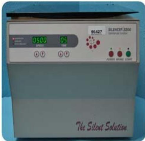
The Silencer® S2200 Centrifuge pictured above is being recalled because there is a potential for the centrifuge to operate with the centrifuge's bucket and insert not properly seated on the rotor which results in the rotor coming loose, breaking the lid and being forced out of the centrifuge. For more information on this recall please visit the following link:
